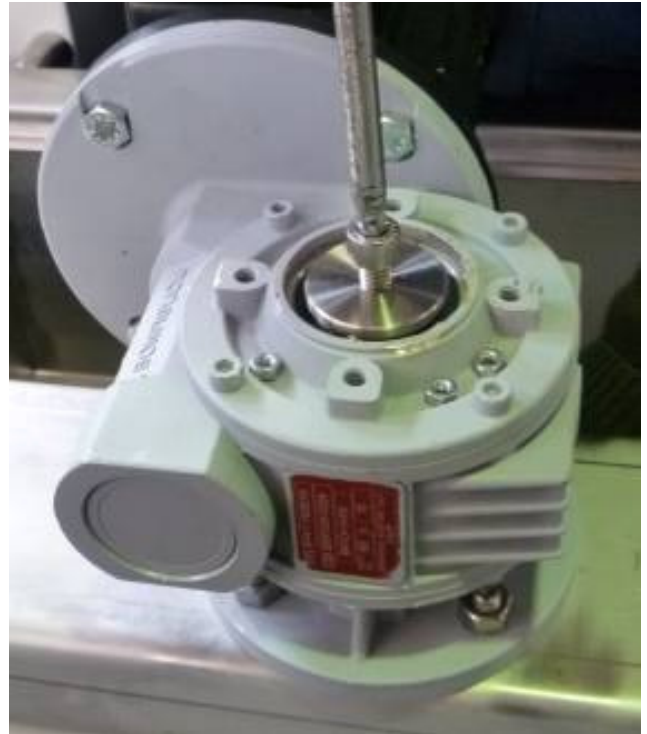
Loosen the bolts located under the protective cover taking care to hold from under the agitator shaft.
