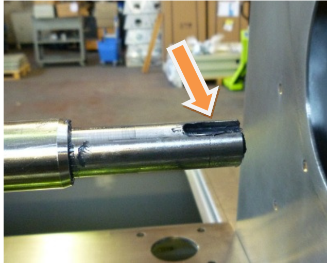
Insert the new part, after lightly greasing the key housing.
