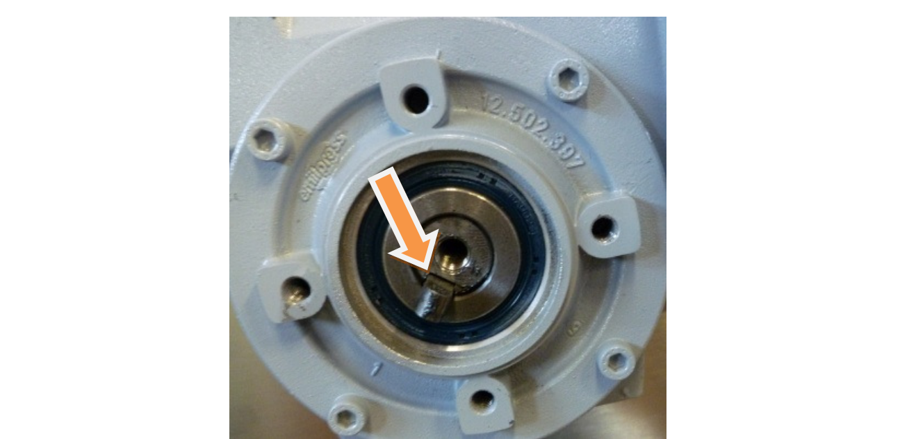
Insert the new part, after lightly greasing the key housing.
