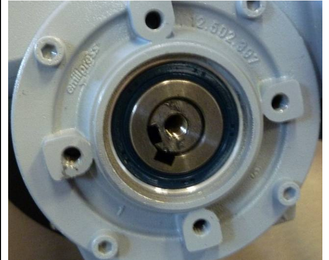
Once the shaft has been inserted, align the two key housings before inserting the key.
