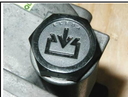
The oil filling plug (pos.119)
