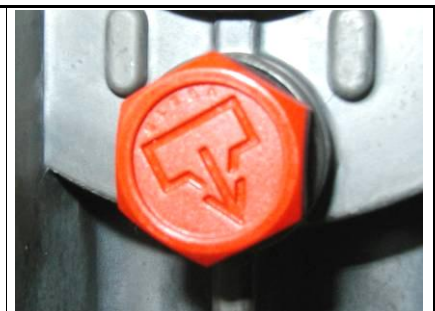
The oil drain plug (pos.121)
