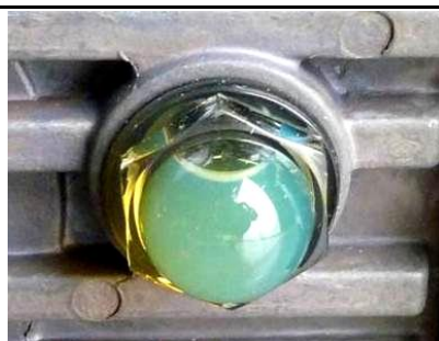
The oil level plug (pos.120)
