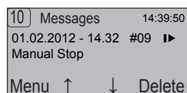
Fig. 48: Display of disturbance messages
