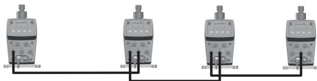
Fig. 31: Synchronization of several dosing pumps by means of stroke feedback and pulse control
