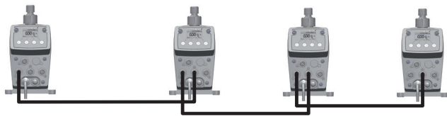
Fig. 18: Synchronization of several dosing pumps by means of stroke feedback and pulse control
